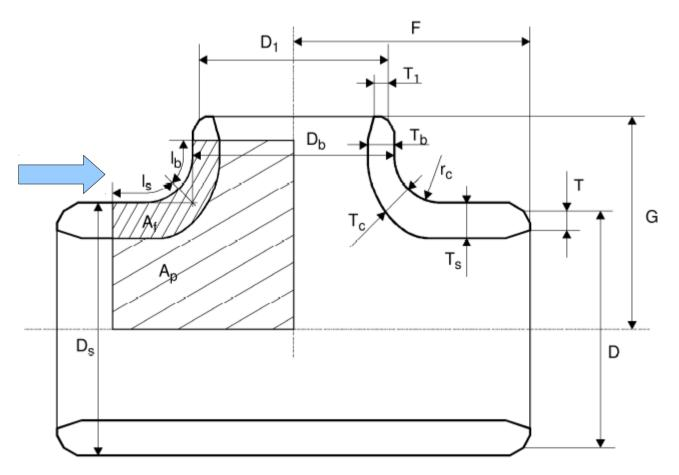
Figure B.5 — Dimensions and areas  $A_p$  and  $A_f$  of a tee
